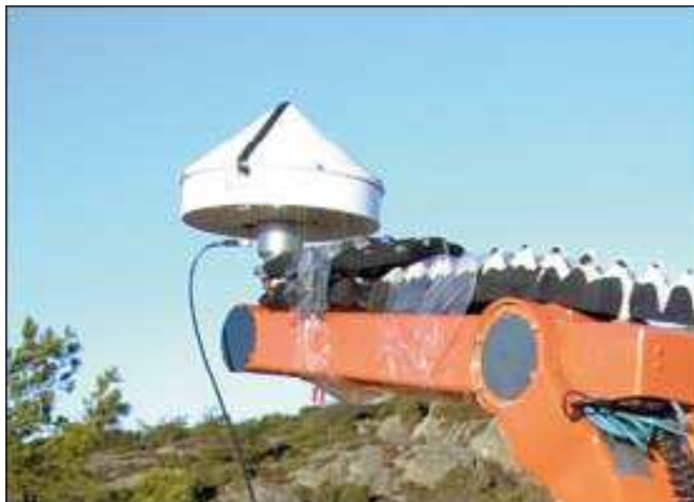
GPS antenna mounted on an industrial robot. The robot is used to simulate movements, such as during seismic events.
